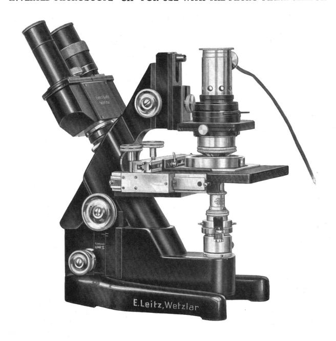
The Microscope "CH" has been constructed according to the suggestion of Professor Robert W. Chambers. By reason of the inverted construction of the microscope, the objective occupies a position beneath the stage, pointing upwards towards the coverglass while the drop of fluid rests upon the latter. Such a construction establishes conditions which greatly favor the technic of micro manipulation.
